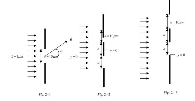
(a)(10) Sketch the diffracted intensity as a function of  $\sin\theta/\lambda$  when a plane wave is incident on a slit as shown in Fig. 2-1. At what value (or values) of  $\theta$  in degrees, the diffracted intensity is zero? Give the  $\theta$  value having the smallest magnitude.
