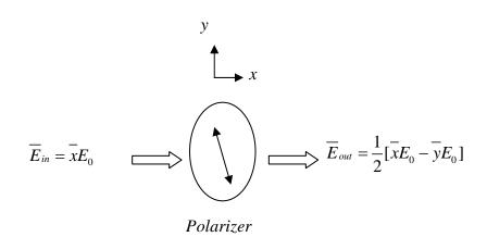
(a)(10) For any input E-field wave, the output of the above polarizer can be expressed as  $\underline{E}_{out} = J \underline{E}_{in}$  where J is a 2x2 matrix. Determine J.
