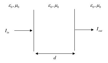
(a)(10) What is  $I_{out}/I_{in}$ ? Give your answer as a function of sin(kd), where k is the wavenumber in the vacuum and d is the distance between two mirrors.
