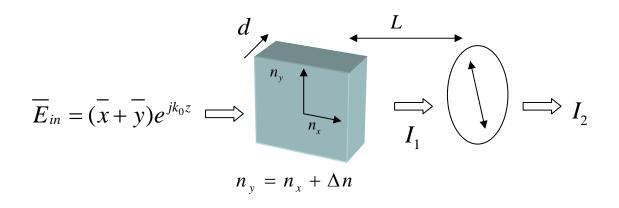
(b)(10) Determine the output intensity,  $I_1$ , after the birefringent material but before the polarizer.
