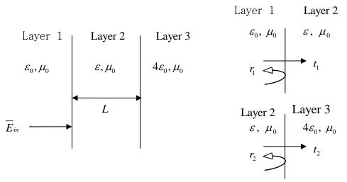
(a) Determine the ratio of transmitted electric field to incident electric field. For your answer, use  $r_1$ ,  $t_1$  and  $r_2$ ,  $t_2$  that are reflection and transmission coefficients for Layer 1,2 interfaces and Layer 2,3 interfaces as shown above.
